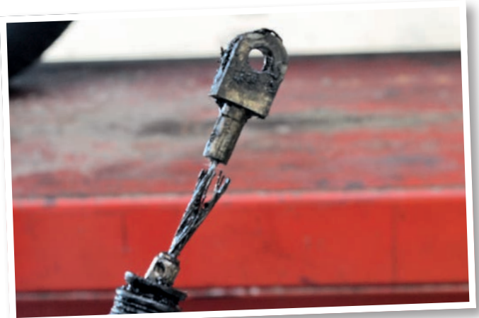
The offending clutch cable
