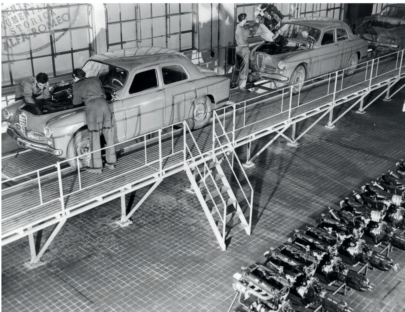
Below Alfa's first real series production model, the 1900, on the line, accompanied by a row of ready to fit engines and gearboxes. Photo, copyright Centro Documentazione Storica Alfa Romeo
