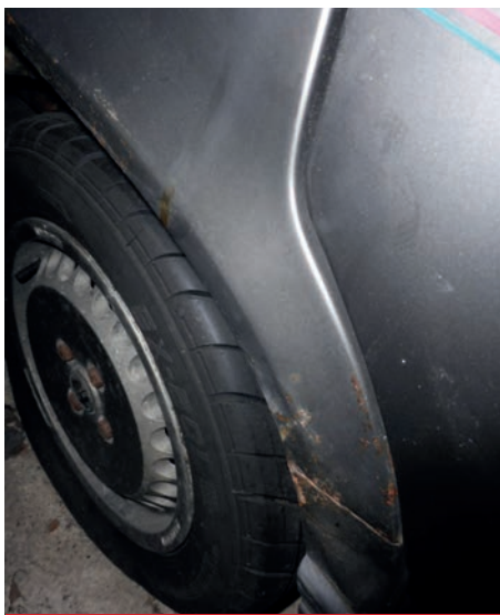
There is rust on the arches
